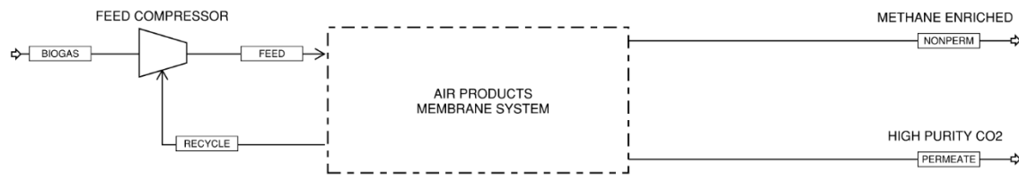
Figure 8. CO 2 Rejection from Gasified Biomass
